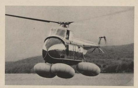
Sikorsky S-55 helicopter makes a simulated emergency landing on water using the new Kidde Inflatair gear. Inflated electrically by the pilot, the doughnutshaped floats can be deflated after initial use, refolded, and then used again.
