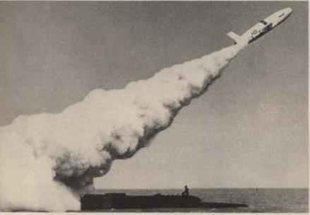
Navy's Chance Vought surface-to-surface guided missile Regulus is launched from the submarine USS Tunny in a test somewhere off the California coast.
