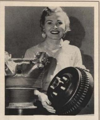
We don't know the name of this month's Breezecake girl, but according to the accompanying release from the Studebaker-Packard Corp. she's holding "the new safety-finned brake for the restyled 1956 model Studebakers." This, the release points out, is an idea borrowed from the aircraft industry. The brake fins, which employ the air-cooling principle, increase the surface area and allow greater heat dissipation. It works the same way as the aircraft engine cylinder does, on the left.
