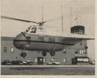
LIFEGUARD FOR TEST PILOTS, Sikorsky S-55 recently purchased by Grumman Aircraft arrives at company's Bethpage, L. I., airfield. Grumman will use the S-55 as a stand-by rescue aircraft while testing its Navy jet fighters off the Atlantic coast. Grumman's S-55 has a 600-pound rescue hoist and flotation gear.
