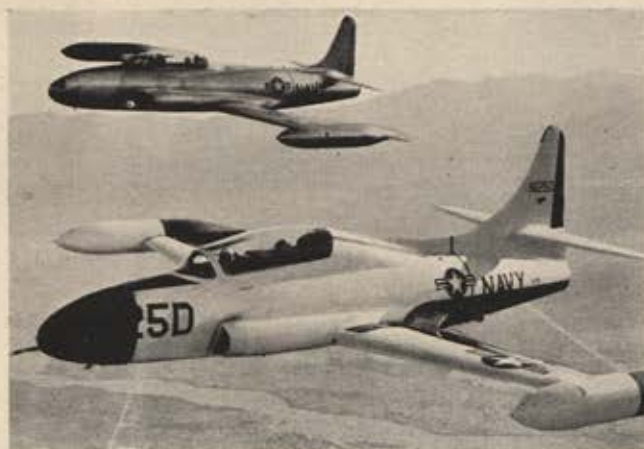
Lockheed T2V-1 (foreground) uses boundary layer control. BLC is one way of reducing take-off and landing speeds.
