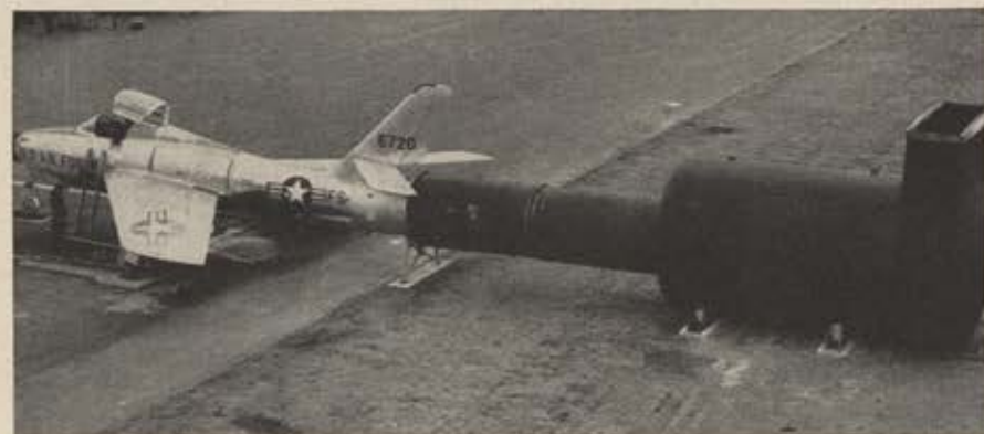
Republic F-84F Thunderstreak is coupled to a new ground muffler which suppresses three-quarters of the fighter's full-power engine noise during tests.
