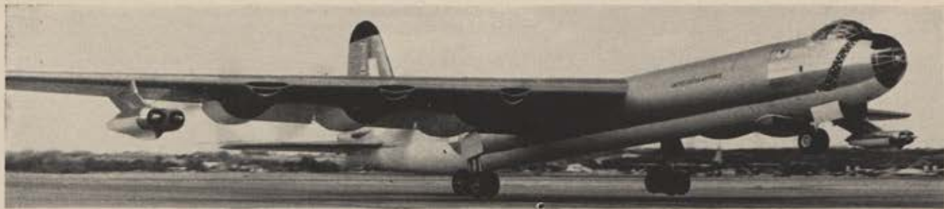
Jet transports will likely use landing gear like that on the B-36 to distribute weight better on existing runways.
