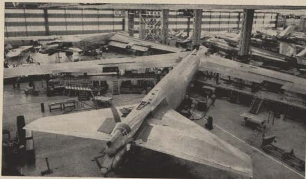
Industrial readiness in action. This is the final assembly area for giant Boeing B-52 Stratofortresses at the Wichita, Kan., plant. The big bombers have also been in quantity production at the Seattle plant since March '54.
