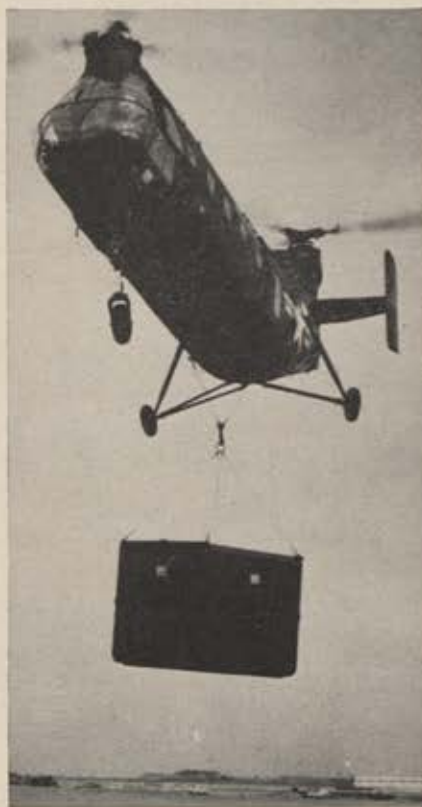
Mobile radio relay station is lifted by Piasecki H-21 helicopter during stability tests at Langley AFB, Va.
