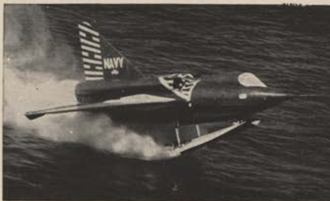
Hydro-skis—one area of research into take-off and landing problems. Above, Navy's Convair XF2Y-1 "Sea Dart."
