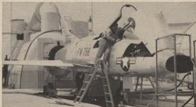
North American F-100 Super Sabre hooked to a noise suppressor. The AF is trying various methods to cut noise.
