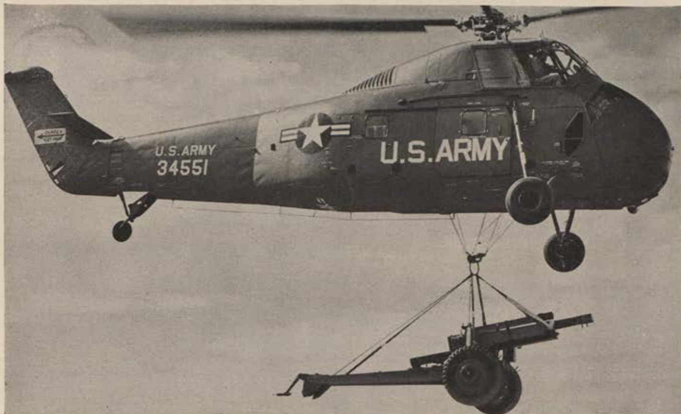
ARMY H-34 CARRIES 2½-TON HOWITZER —At Fort Sill, Okla., a big Sikorsky H-34, newest member of the Army aviation family, carries a 105mm howitzer. This was the
