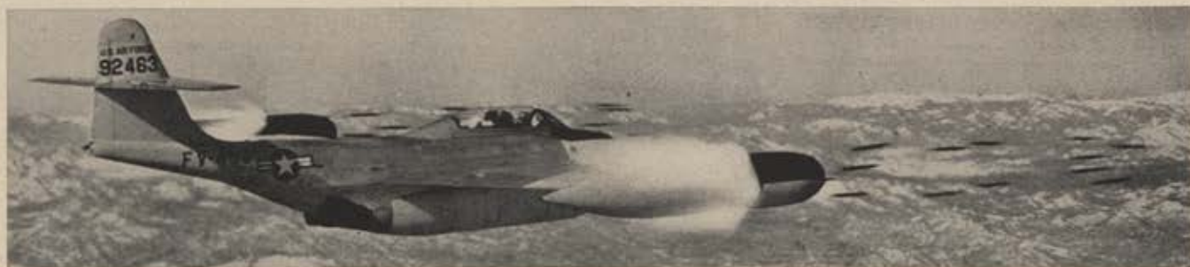
All Continental Air Defense Command planes are loaded when on missions. Northrop F-89D Scorpion carries 104 rockets.
