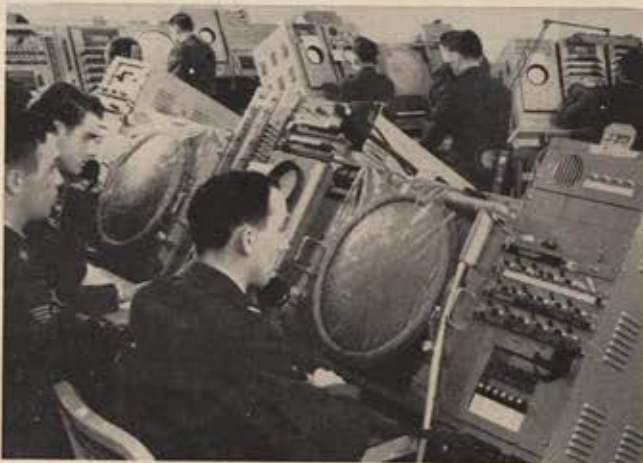
Display consoles of the Whirlwind I. This digital computer is one of the highest performing in existence and can quickly process large quantities of air defense data.
