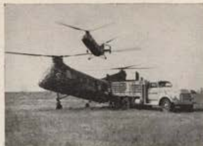
For rapid cargo transport, large trucks can be unloaded directly into the cabin through two doors without stopping rotors.
