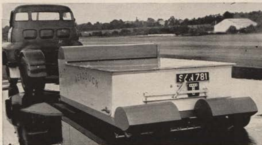
The "Aeroduck," manufactured by Comex-Fraser Tuson Ltd. of London, blots up hazardous pools of water from runways. It can soak up 400 gallons in minutes.
