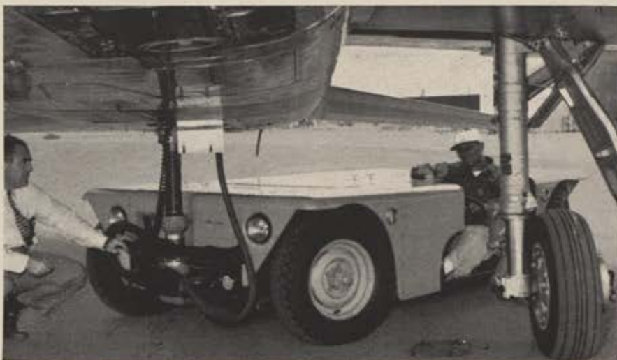
Mechanical starter developed by North American Aviation can drive under low-slung jets. It was designed by North American engineer Dan Coleman, left.
