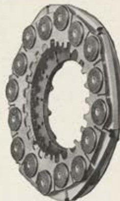
Cerametallic lining attached to brake stator.
