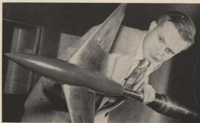
Richard T. Whitcomb inspects a model incorporating his new "area rule" shape. Note contour at the wing roots.
