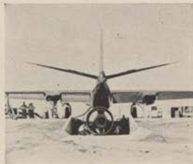
Flying test beds like this B-45 airplane are used to test new designs in the air . Flight testing is the ultimate proof of the value of a new design.
