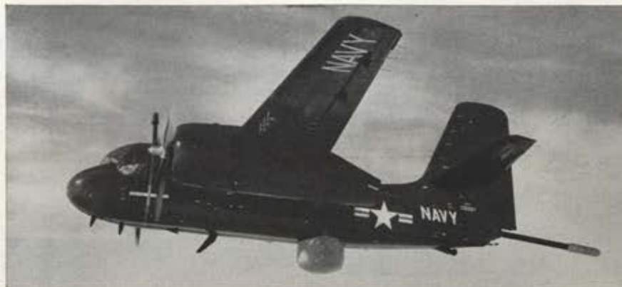
Grumman S2F carries radar and a magnetic boom for detecting submerged subs.
