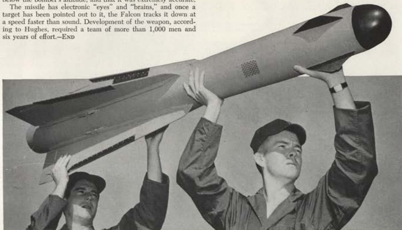
The six-foot, 100-pound Falcon is the smallest guided missile in production. It can be carried in small fighters.
