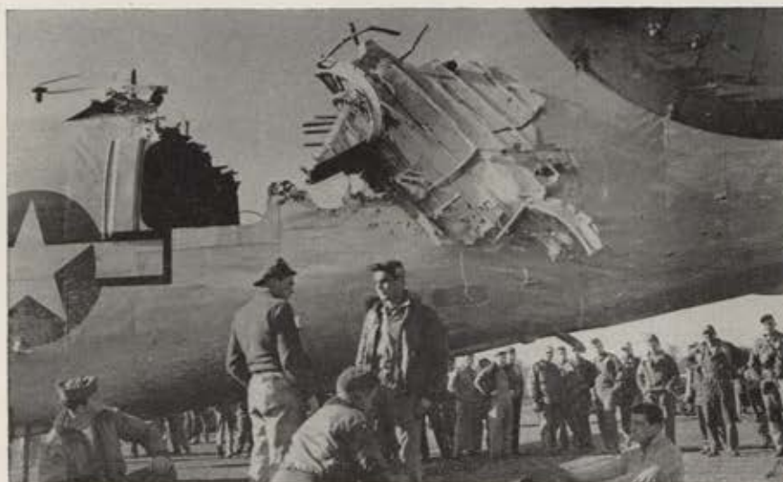
A direct flak burst over Yugoslavia chopped this gaping hole and severed the plane's rudder controls, but the 15th AF B-24 Liberator made it back to Italy.
