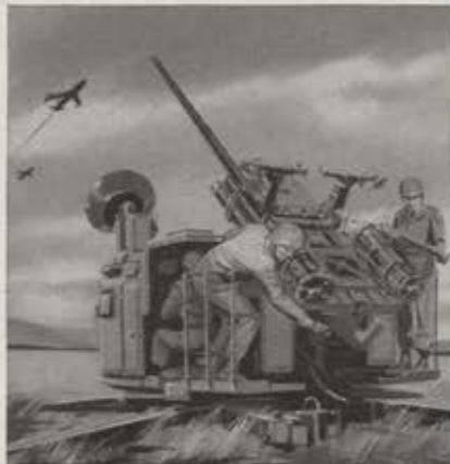
T-38 SkySweeper, self-aiming anti-air- craft gun.
