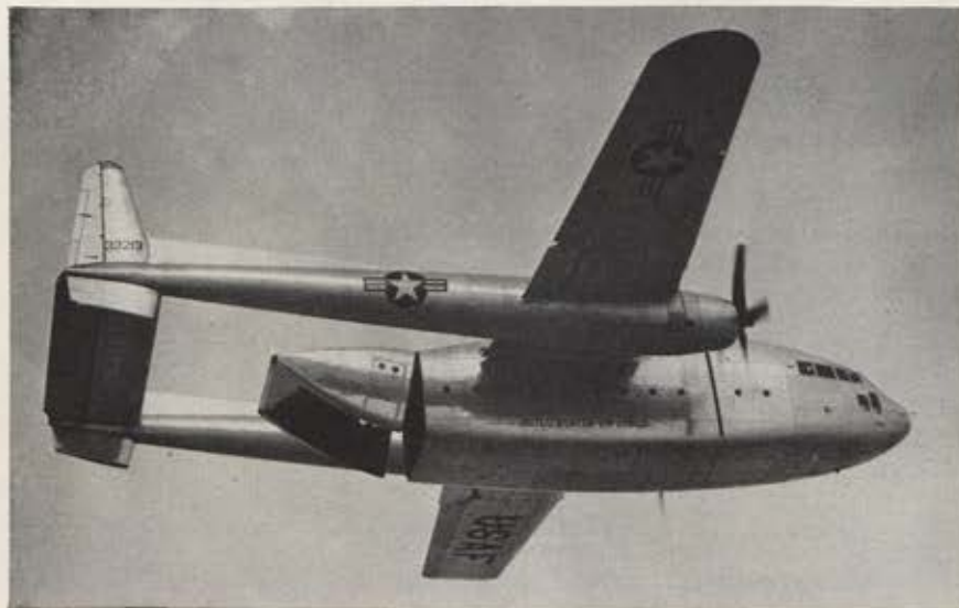
A new flight-opening cargo door is being flight-tested on a Fairchild C-119.
