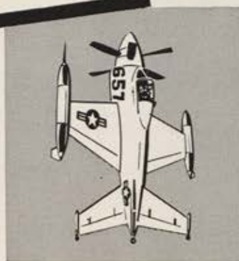
LOCKHEED XFY-1 vertical take-off fighter for the U.S. Navy
