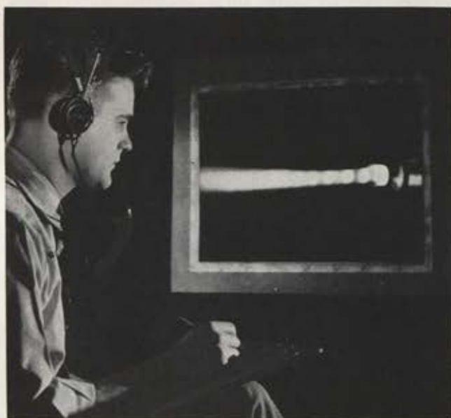
NACA engineer at Lewis Laboratory, Ohio, studies shock waves of a thrust augmentation bleed-off turbojet engine.
