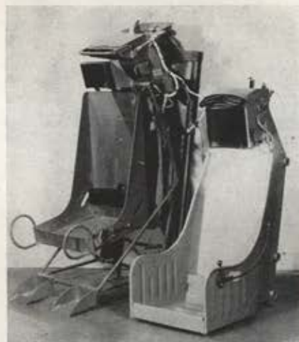
Present F7U-3 seat (left) weighs 130 lbs. New one weighs only thirty lbs.
