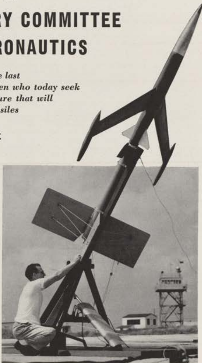
Typical of NACA's research projects is this rocket model. The technician is checking the model's external booster.
