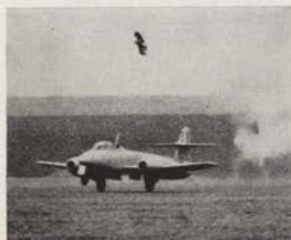
A life-size dummy is ejected at ground level at speed of 130 mph.
