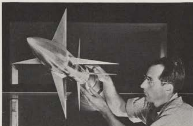
Missile design problems are studied in the supersonic wind tunnel at NACA's Ames Laboratory in California.
