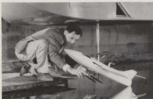
An NACA engineer readies a dynamic model equipped with hydro-skis for a test run in the Towing Tank at Langley.
