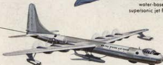
GRB-36 "AIRCRAFT CARRIER" — launches and retrieves fighters in flight
