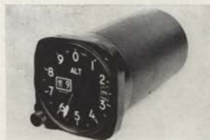
An altitude of 9,565 is shown on Kollsman's new altimeter. Two digit counter registers thousands of feet.
