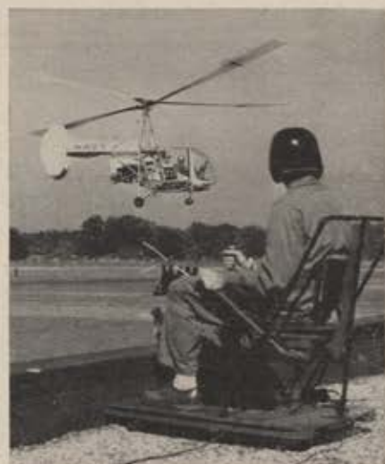
Kaman Aircraft's remote-controlled helicopter, developed for the Navy.
