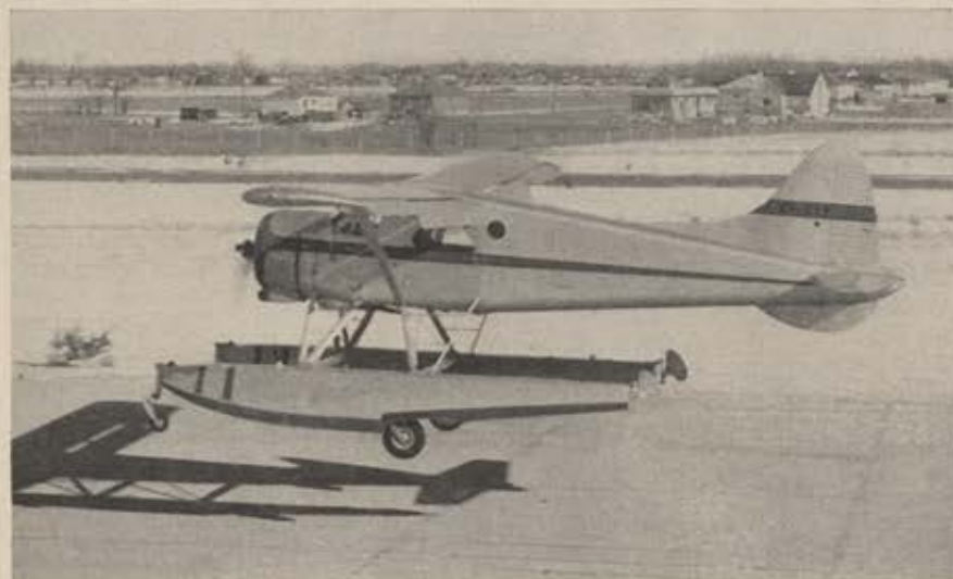
Floats on de Havilland's "Beaver" use wheels and brakes for runway operation.
