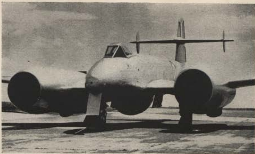
Deflectors, seen below engines, lower stalling speed of this Gloster Meteor.
