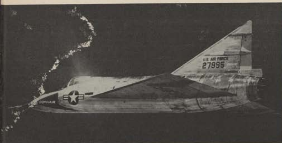
A Pratt and Whitney J-57-11 turbojet powers this supersonic Convair F-102.
