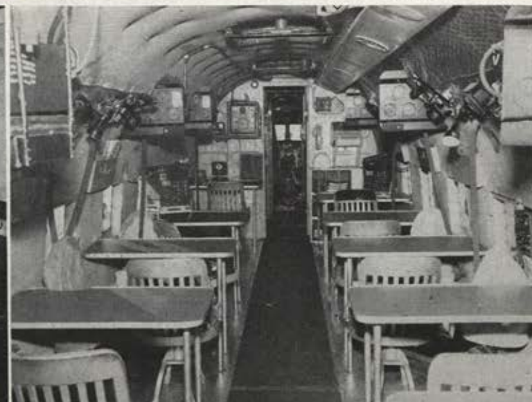
Interior of the TC-47. The trainer has nine navigator positions, each with its own instruments, plus three Loran stations, astrodomes, other gear.
