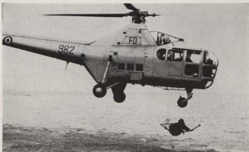
This net was developed by Britain's Royal Navy to rescue injured or unconscious survivors who might be further injured by use of conventional sling.
