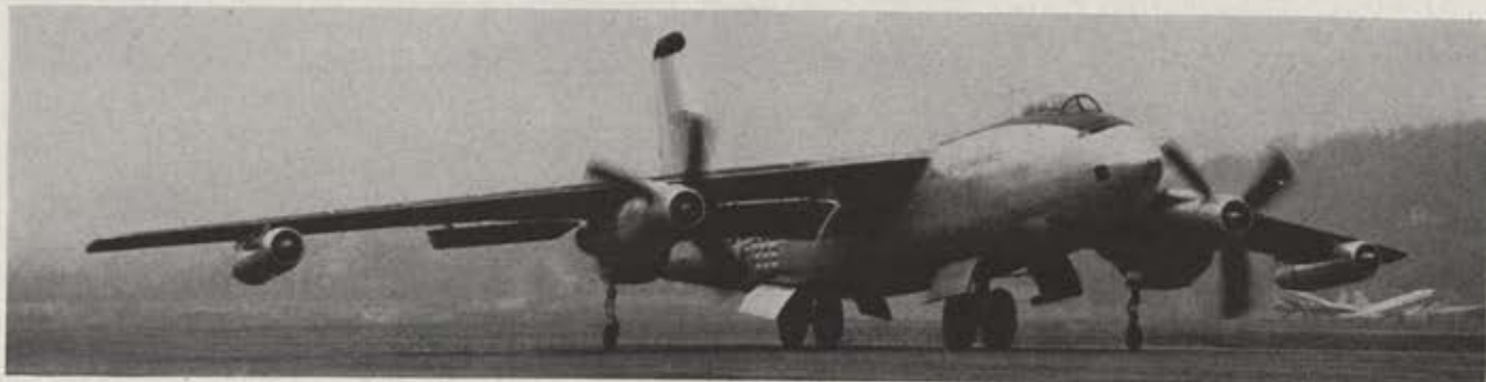
This jet-prop combination is a Boeing XB-47D, a standard B-47B modified to test the Curtiss-Wright T-49 turboprop engine. The engines are mounted in place of the four General Electric J-47 turbojets at the inboard pod positions.
