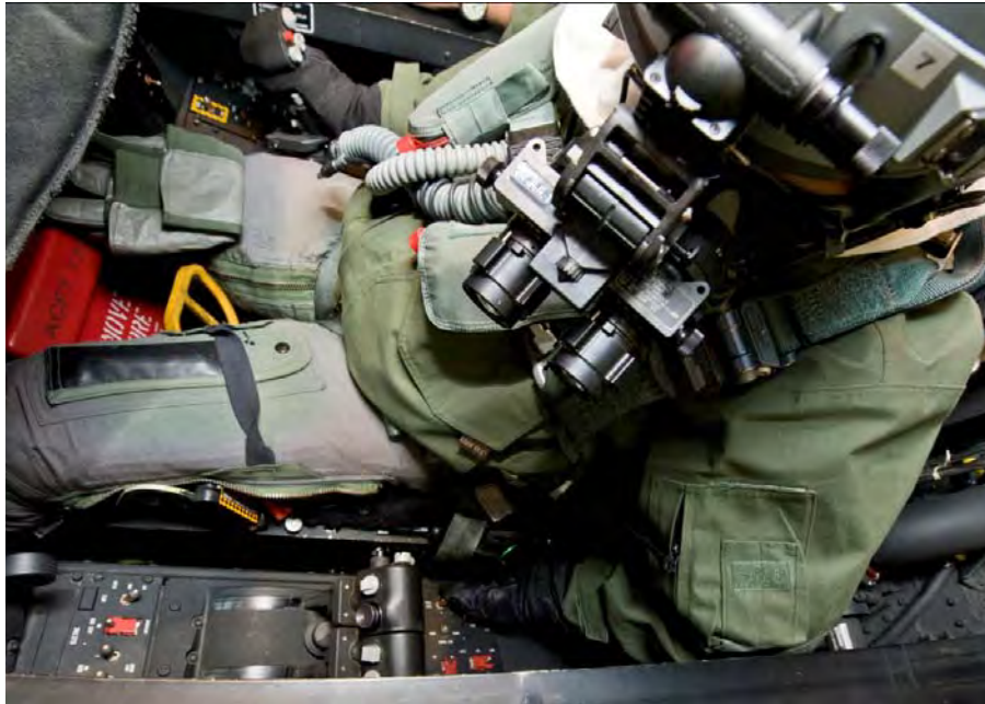
Figure 15 - Pilot pulling EOS activation ring. NVG interfering with EOS ring visualization. (Tab CC-5 and Tab Z-7)
