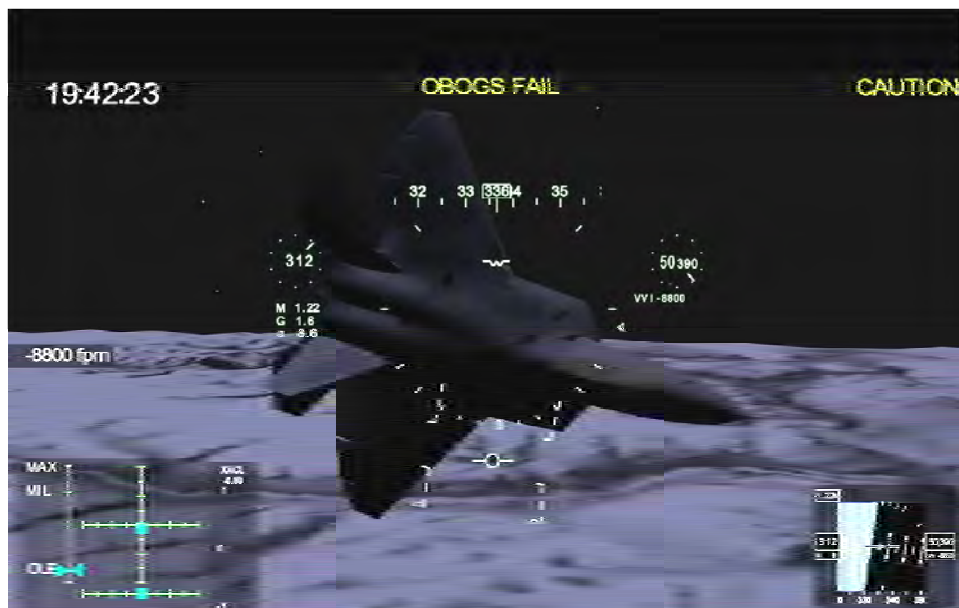
Figure 3 19:42:23 – MA parameters at assertion of OBOGS FAIL caution ICAW. (Tab EE)
