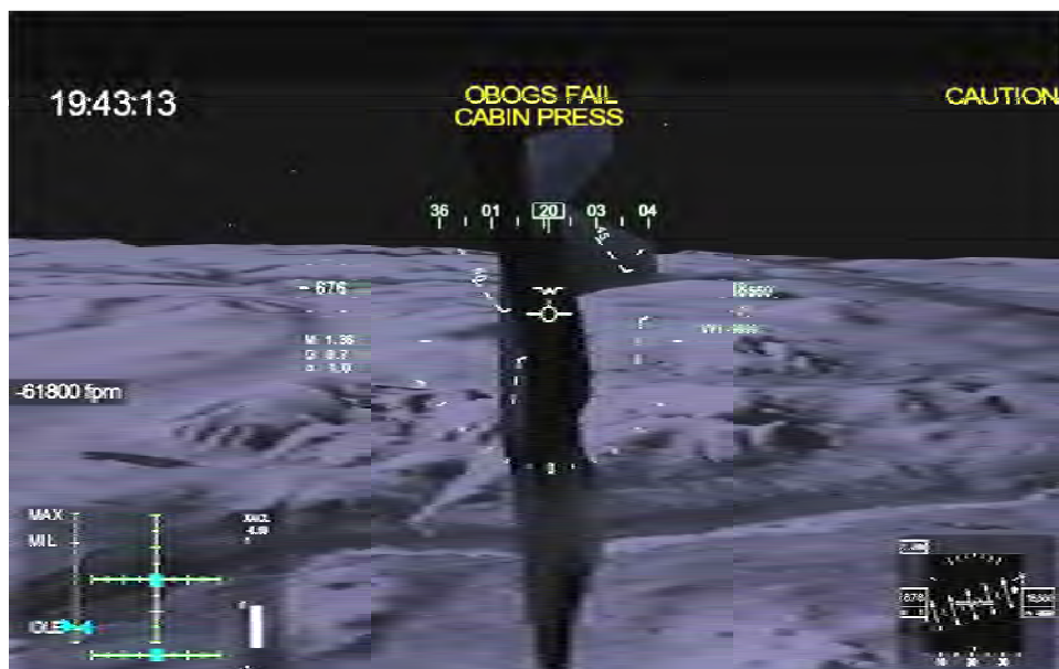
Figure 8 19:43:13 – MA parameters at assertion of CABIN PRESS caution ICAW. No stick or pedal inputs. (Tab EE)
