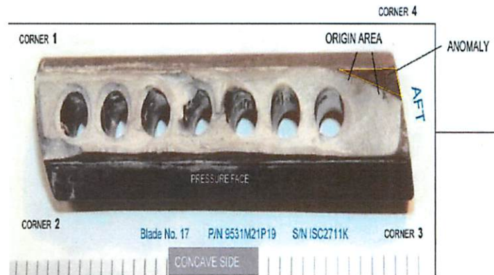
Figure 9. Dovetail View w/ Anomaly (Tab J-41) Figure 10. Dovetail View from Broken Blade Side (Tab J-36)
