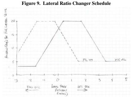
**Note:** The X-axis is longitudinal stick position in inches; Y-axis is the aileron deflection in degrees; The dashed lines is the schedule with the PTC nose-up (NU), solid line is the schedule with the PTC nose-down (ND). (Graph and information provided by Boeing SME)
