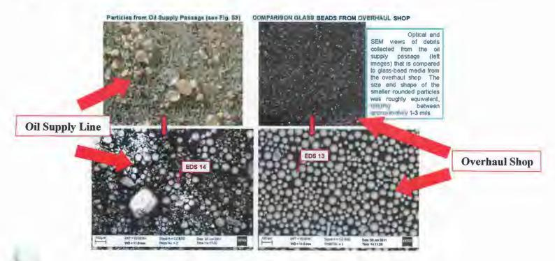
Figure 17: Glass-Bead Media (Tab J-103) F-16C+, S/N 87-0242, 7 June 2011 In addition, a piece of white debris consistent with Teflon<sup>®</sup> was found that was approximately 223 millimeters long by 44 millimeters thick and 82 millimeters wide (Figure 18) (Tab J-37 and J-102).
