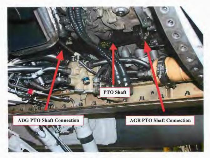
Figure 9: ADG to AGB connection (Tab Z-4)
