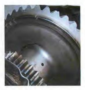
**Figure 8: PTO Shaft Bevel Gear**
