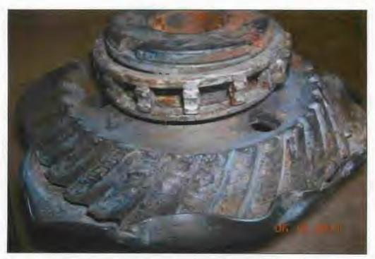
Figure 13: Bevel Gear Teeth (Tab J-19)
