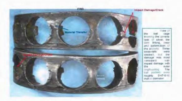
Figure 15: Ball Bearing Cage (Tab J-78)
