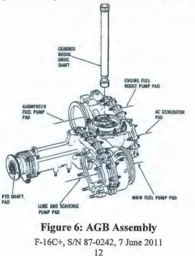
Post-mishap analysis was performed by General Electric Aviation and Tinker OC-ALC Engineers (Tab J-23). The recovered parts were analyzed at the 115th JEIM shop (Tab J-3). Engineering analysis determined that the PTO shaft forward ball bearings were reduced in size allowing PTO shaft movement (Tab J-82). The PTO shaft movement ultimately resulted in disengagement of the mating bevels gears (Figure 7) within the AGB (Tab J-16).
