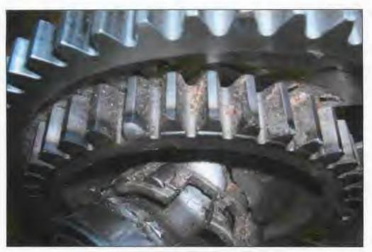
Figure 12: PTO Spur Gear Teeth (Tab J-18)
