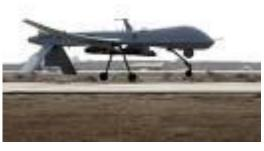
and maintenance personnel for deployed 24-hour operations. The basic crew for the MQ-1B Predator is one pilot and one sensor operator. They fly the MQ-1B Predator from inside the GCS via a line-of-sight (LOS) radio data link and via a satellite data link for beyond LOS flight. A ground data terminal antenna provides LOS communications for takeoff and landing while the PPSL provides beyond LOS communications during the remainder of the mission. (Tab Z-7)
