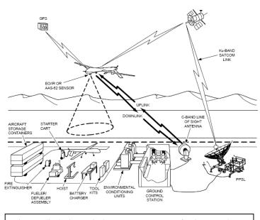
Diagram displaying typical system components of MQ-1B Predator
