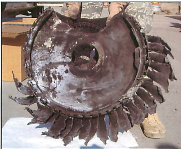
Engine's Second Stage Fan Disk Following Removal
