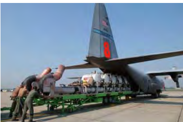
Airmen from the North Carolina Air National Guard's 145 th Airlift Wing push a modular airborne fire fighting system onto a C-130 Hercules. The system is a series of pressurized tanks that hold 3,000 gallons of flame-retardant liquid. The retardant is dropped along the leading edge of a fire to block the spread of flames.
