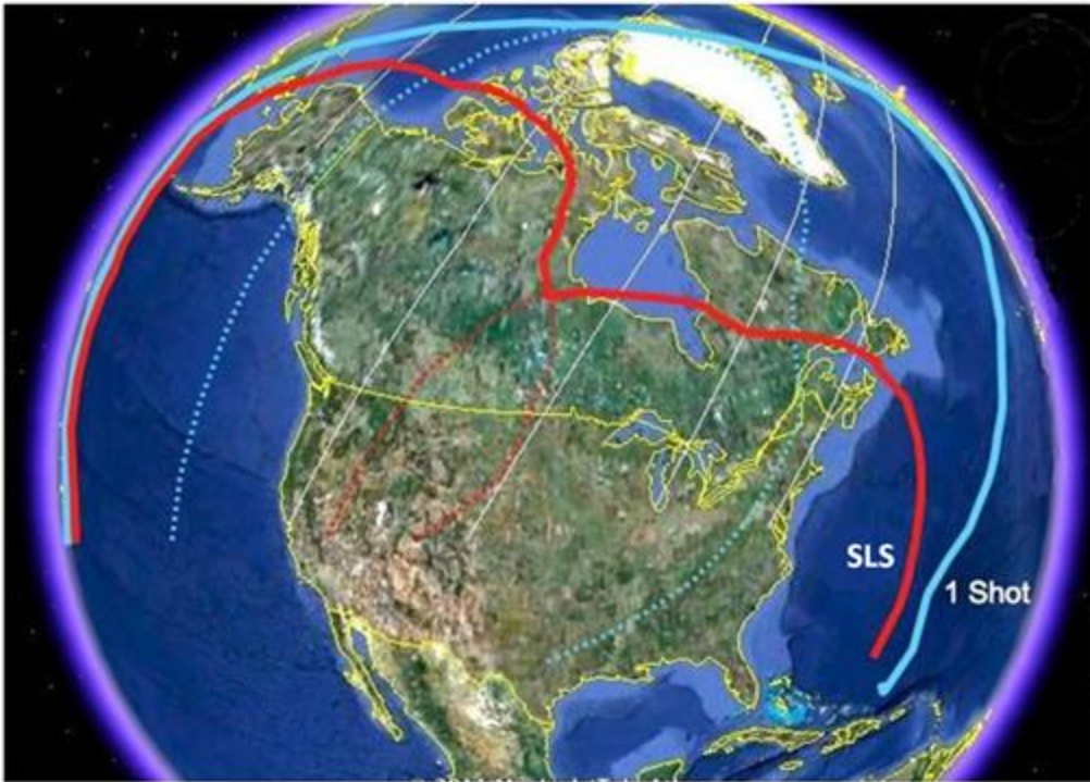
FIGURE 5-9 Notional single-shot and SLS footprints against minimum energy ICBM trajectories from Iran.
