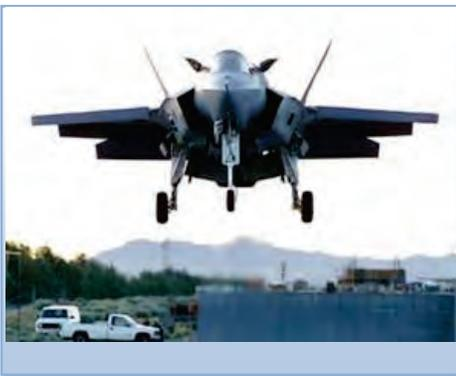
The **F-35B** is the Short Takeoff and Vertical Landing (STOVL) fighter, which will be used by the U.S. Marine Corps (USMC). The beddown of F-35B training and operational aircraft is addressed in environmental documentation prepared by the USMC.
