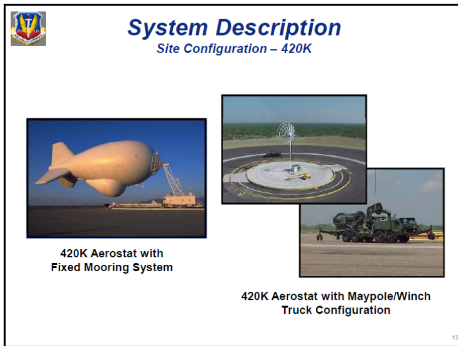
Figure 2b. 420K Site Showing Winch Truck Configuration. (Tab II-24)
