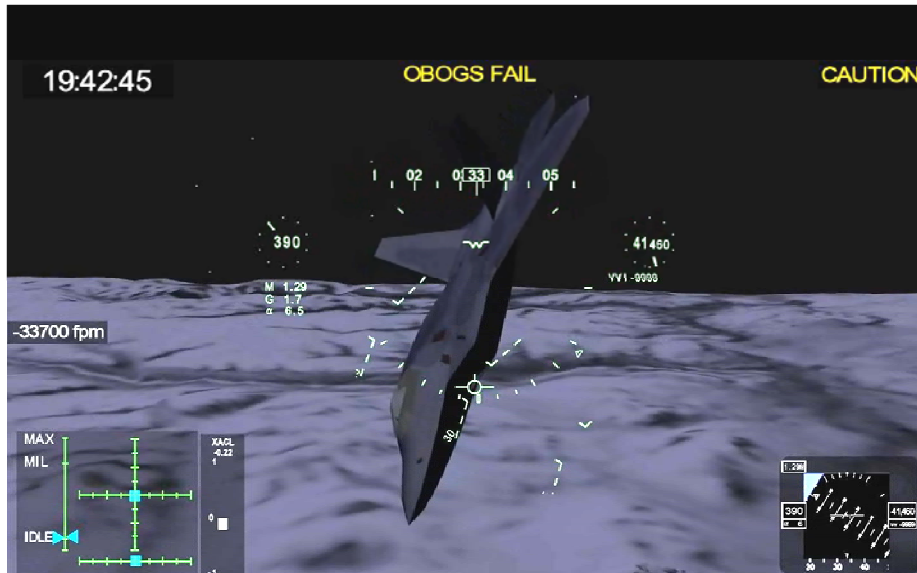
Figure 4 19:42:45 – MP deliberately flew to a controlled attitude of 30 degrees ND and 44 degrees RWD in order to descend to a lower altitude IAW the checklist. (Tab EE)
