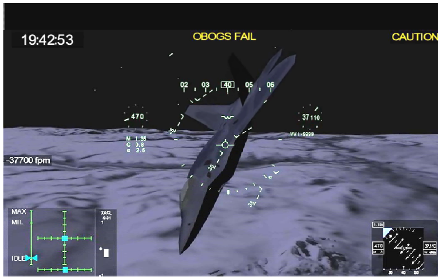
Figure 5 19:42:53 – MA parameters after 8 seconds of zero MP inputs to stick, pedals, or throttles. (Tab EE)
