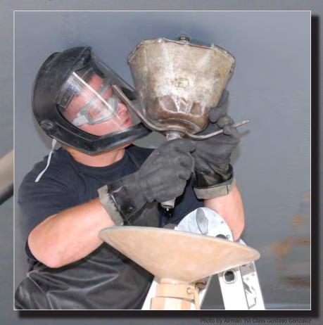
Senior Airman Neal Sicard, 340th Aircraft Maintenance Unit crew chief, preps for maintenance work on the KC-135 Stratotanker fuel cell by draining the main fuel tank sumps.
