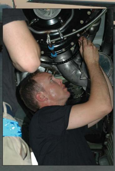
Staff Sgt. Kevin Tarwater, electronic warfare systems craftsman with the 55th Aircraft Maintenance Unit, replaces an air cycle machine which is used as one of the primary means to cool the aircraft cabin.
