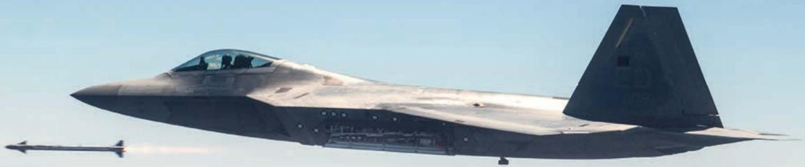
**An F-22 releases an AIM-9X from its weapons bay in a recent test. The AIM-9X and AIM-120D are two key elements of the Increment 3.2 Raptor upgrade.**
