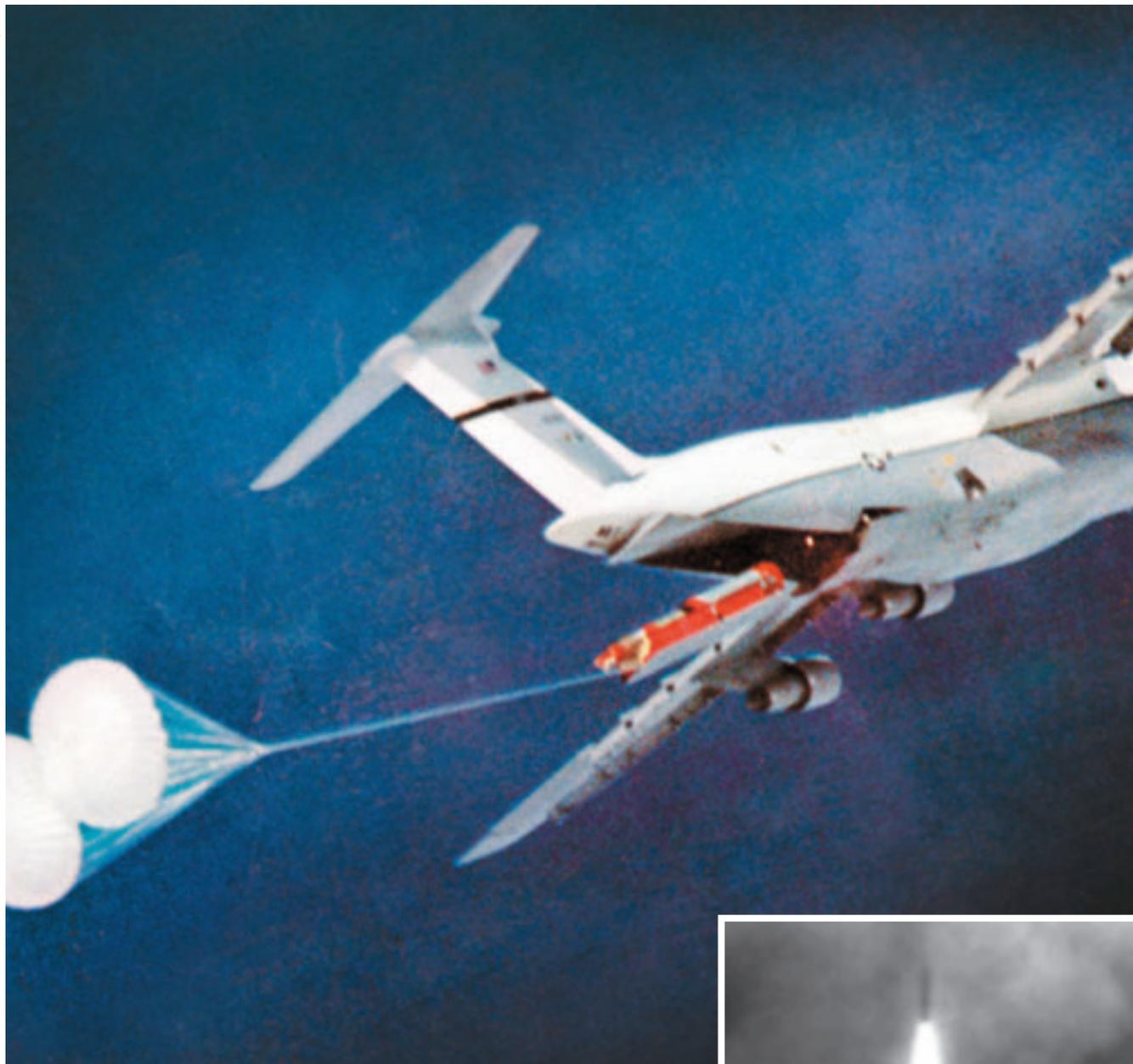
By 1970, increasingly accurate Soviet ICBMs had begun to pose a threat to silo-based US nuclear missiles. Thus began a search for more survivable basing. One idea was an "air-mobile ICBM," which actually was tested. On Oct. 24, 1974, USAF sent up a C-5 stuffed with a 60-foot-tall, 86,000-pound Minuteman. The C-5 carried the ICBM to 20,000 feet above the Pacific. The rear cargo bay
