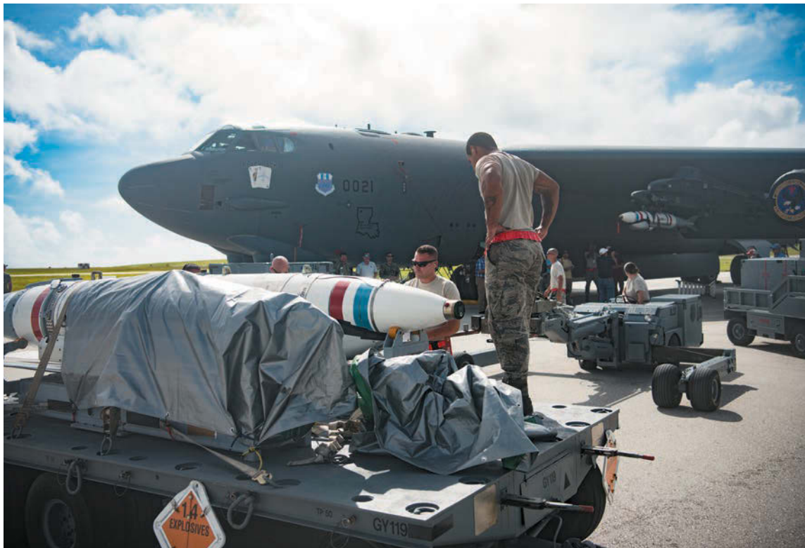
Airmen prepare to load a Quickstrike-Extended Range mine onto B-52s at Andersen AFB, Guam. BUFFs are expected to remain in service through 2050, completing some 100 years of service.
