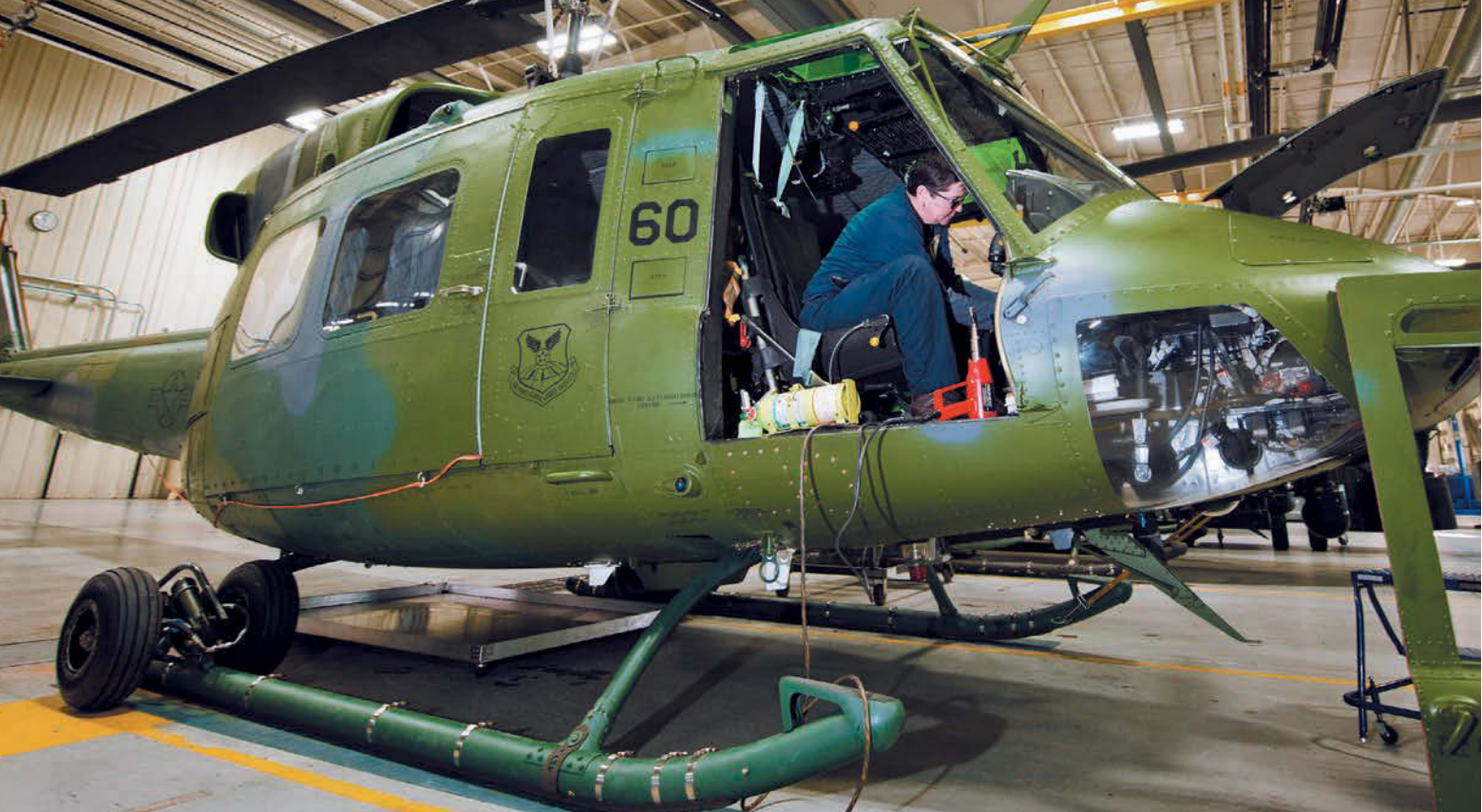
Kim Smith, a 54th Helicopter Squadron UH-1N mechanic, rewires an attitude director indicator in a hangar at Minot AFB, N.D., in January 2017. The replacement of this 1970s-era aircraft has taken a detour through legal limbo.
