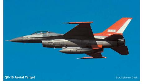
Electric F110-GE-100 turbofan, 28,984 lb thrust. Accommodation: Safety pilot (optional) on ACES Il zero/zero ejection seat.
