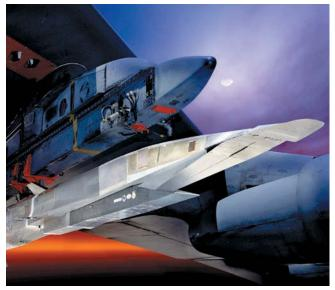
The X-51A Waverider, shown here tucked under the wing of a B-52, will demonstrate hypersonic flight.
