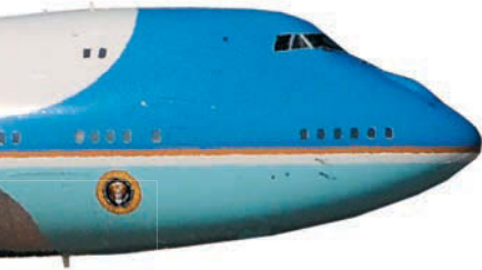
VC-25 is a specially configured Boeing 747-200B known as Air Force One when transporting the president.
