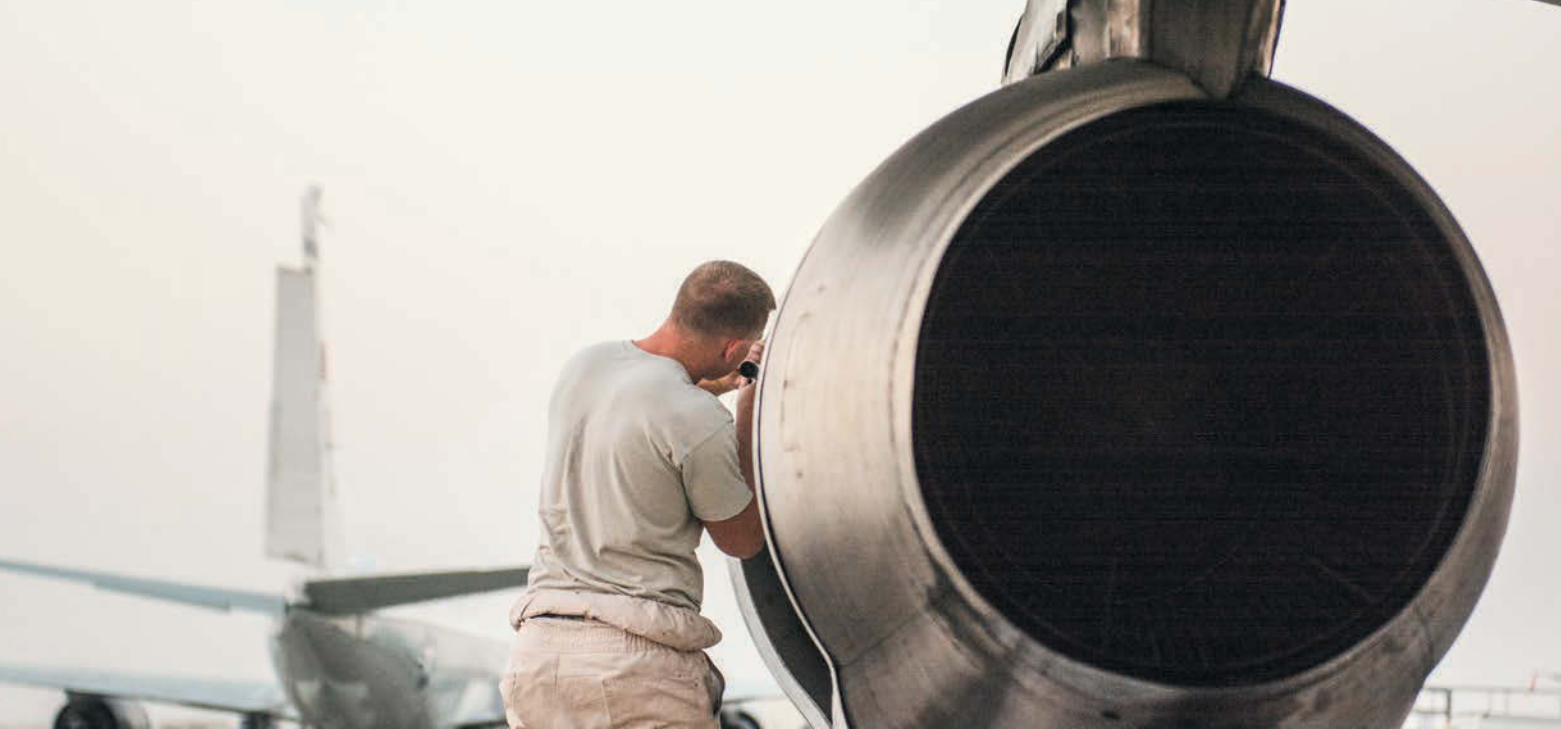
SSgt. Daniel Spear runs through a postflight inspection of the intake and exhaust system on an E-8C JSTARS at Al Udeid.
