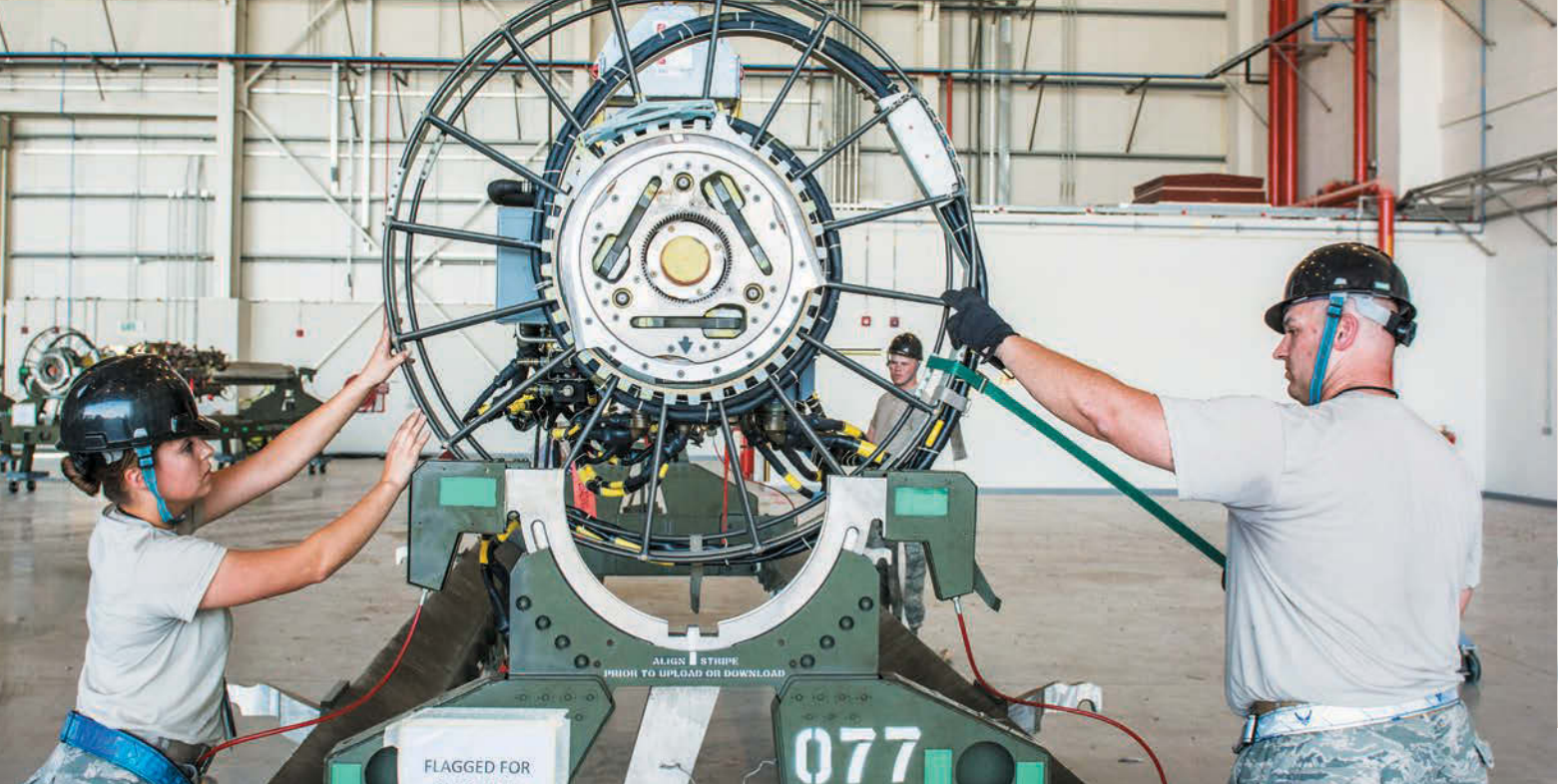
SRAs Chelsie Malloy (left) and TSgt. Dustin Hyden ready a B-52 conventional rotary launcher for transport at Al Udeid.
