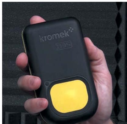
A Kromek handheld radiation isotope detector. The devices provide real-time data to detect radiation.
