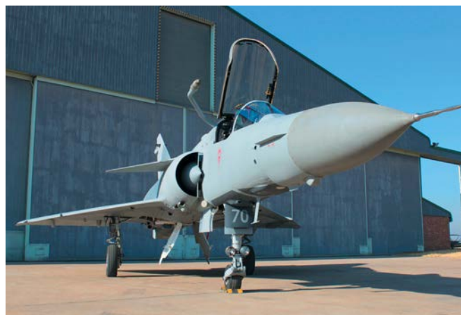
Draken bought 12 South African air force Cheetah aircraft. The Mirage variants are young, with an average of 500 flight hours per airframe and can fly Mach 2.
