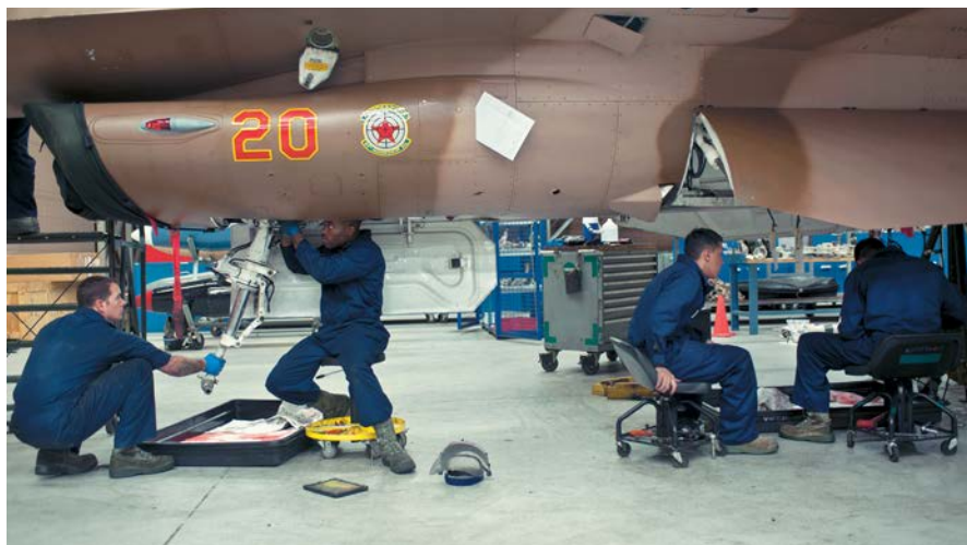
F-16 maintainers replace the landing gear on an Aggressor F-16 at Nellis in 2015.
