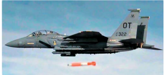
A B61-12 test unit is dropped from an F-15E during a development flight test in 2015.
