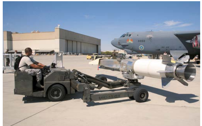
SSgt. Jonathan Young prepares to upload the X-51A WaveRider hypersonic flight test vehicle to a B-52 for fit testing at Edwards AFB, Calif.
