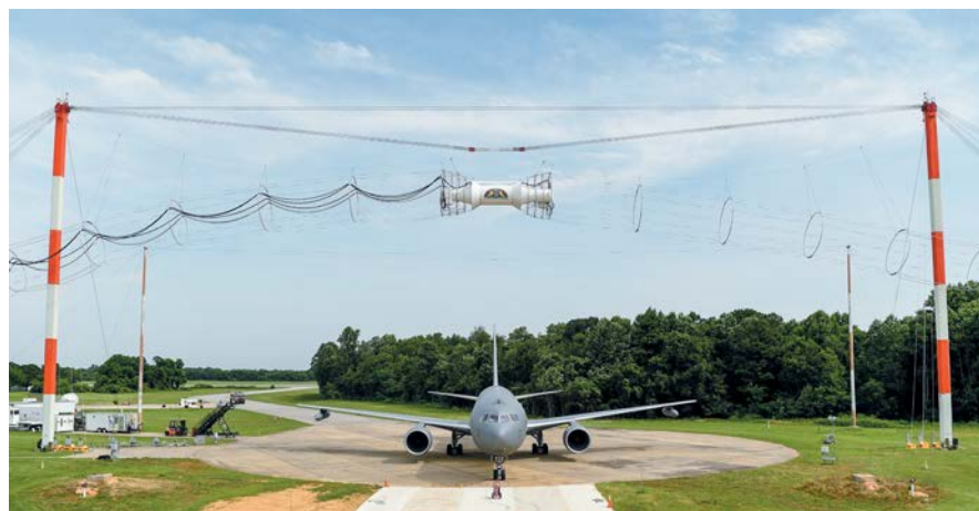
A Pegasus undergoing tests on the electromagnetic pulse pad at NAS Patuxent River, Md., in July 2017.
