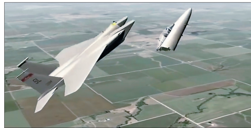
Image from a video produced by Boeing as part of the Air Force’s accident investigation reconstructing the in-flight structural failure of an ANG F-15C in November 2007. The breakup was caused by fatigue cracking of a forward fuselage longeron; the pilot survived.
