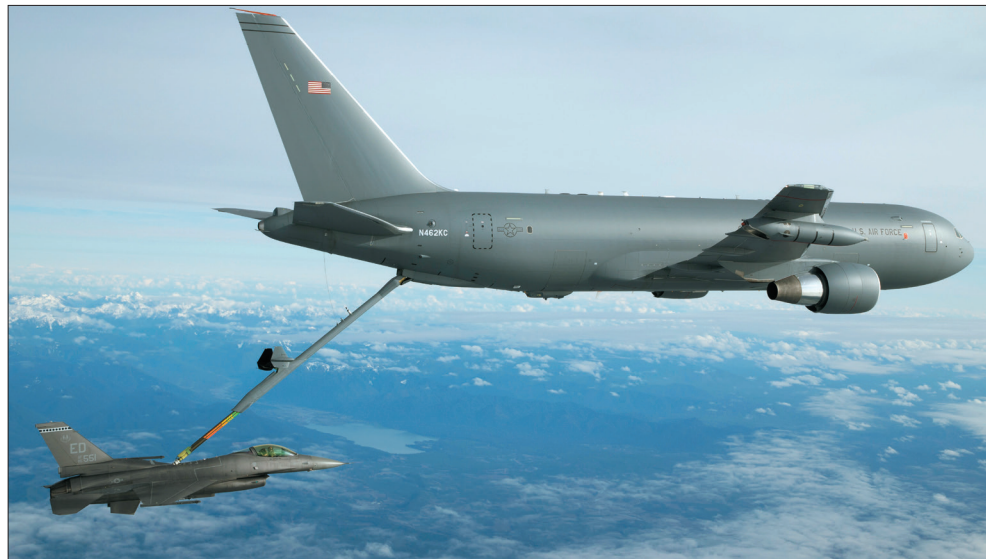
KC-46A fuels an F-16 during tests in January 2016.
