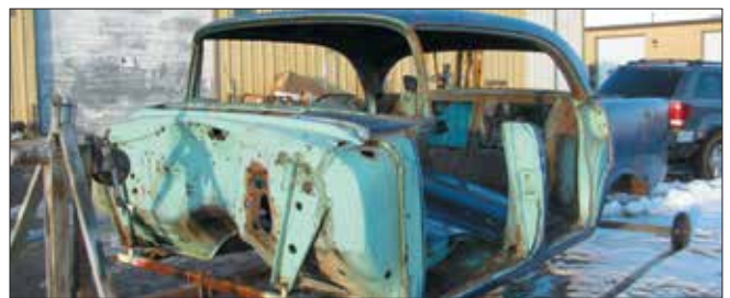
Starting from scratch: This 1956 Chevy is about to be sand blasted down to bare metal.
