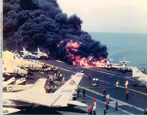
During the Vietnam War, a malfunction caused a Zuni rocket to fire from an F-4 on the deck of USS Forrestal. Leaking fuel and exploding bombs killed 134 sailors. Afterward, training for the possibility of a flight line fire became standard.
