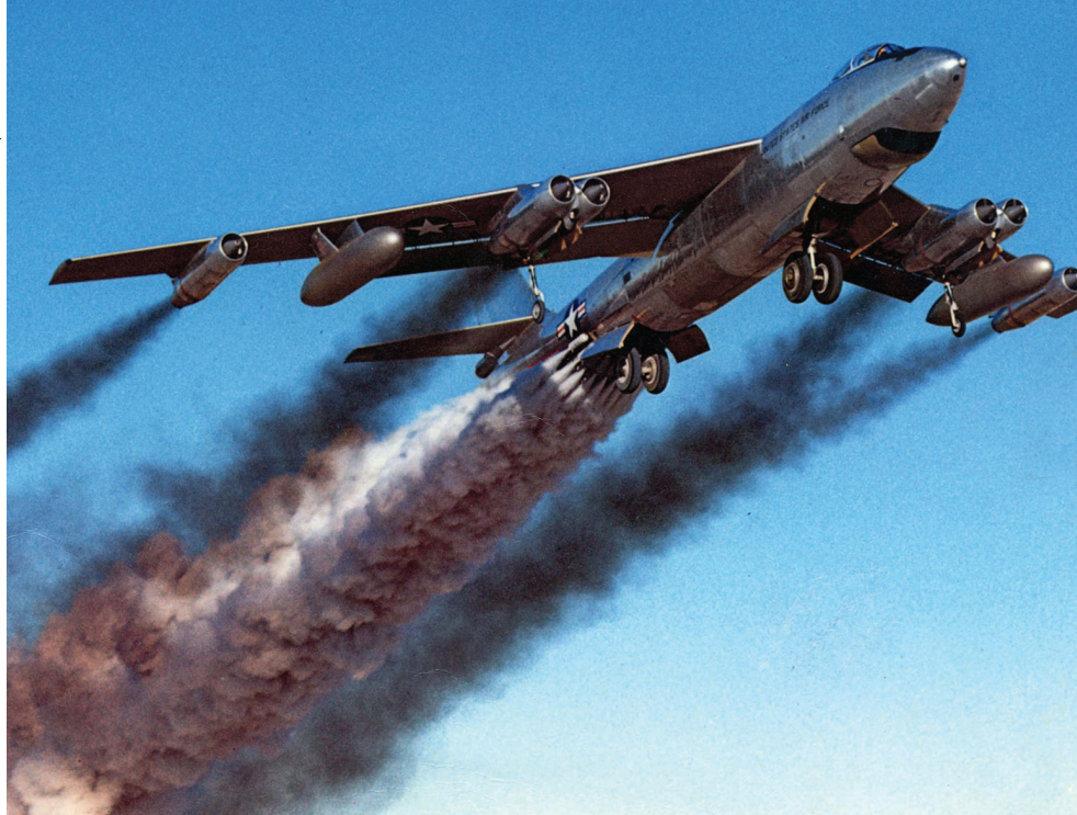
A B-47B makes a rocket-assisted takeoff on April 15, 1954. US bombers and missiles helped keep the Soviet Union at bay for decades.
