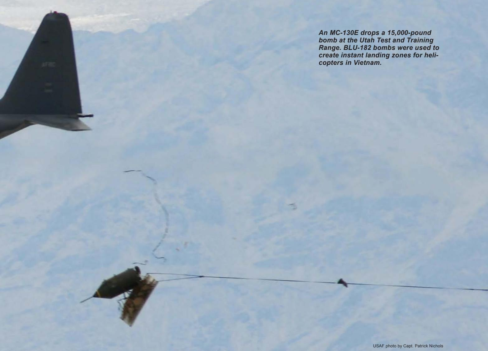
*An MC-130E drops a 15,000-pound bomb at the Utah Test and Training Range. BLU-182 bombs were used to create instant landing zones for helicopters in Vietnam.*
