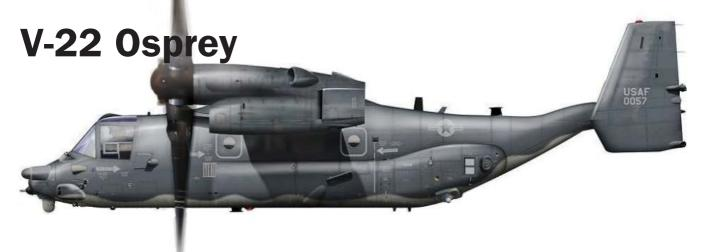
The V-22 Osprey "tilt-rotor" is a unique multimission aircraft capable of vertical and short takeoff and landing. Typically, it takes off and lands like a helicopter. However, when airborne, its engine nacelles and 38-foot, three-bladed proprotors can rotate forward 90 degrees for horizontal flight, converting the Bell Boeing aircraft into a more fuel-efficient, higher-speed turboprop aircraft.
