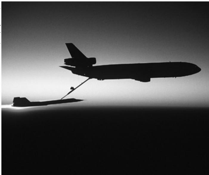
A KC-10 Extender refuels an SR-71 Blackbird in-flight during testing.
