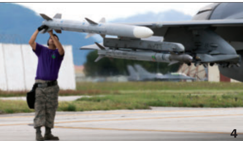
/1/ Armed with M16s, SSgt. Maurice James (left) and A1C James Oshel, security forces airmen, stand next to a Humvee with a roof-mounted weapons station while providing security for an F-16 at Aviano. /2/ Capt. Matt Robbins, a 510th FS pilot, checks an AIM-9 Sidewinder missile as part of his preflight check. /3/ A four ship from the 31st FW flies over Venice, Italy, on a training flight southwest of their base. /4/ SrA. Enrique Melgarejo performs an end-of-runway preflight check on an AIM-120 AMRAAM as an F-16 prepares for a flight.
