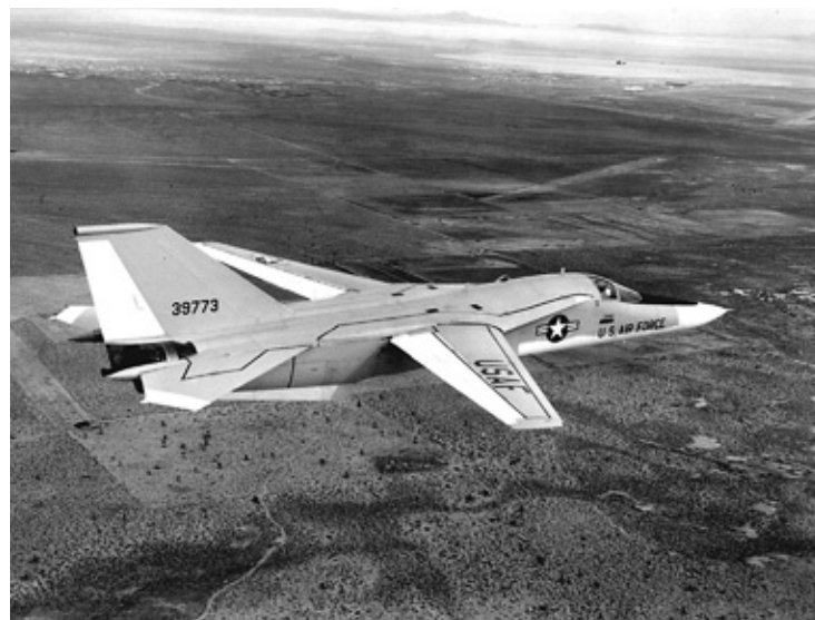
An F-111A with wings forward for lower-speed flight.
