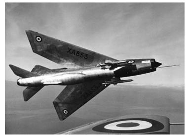
A banking Lightning displays a pair of Firestreak infrared guided missiles.
