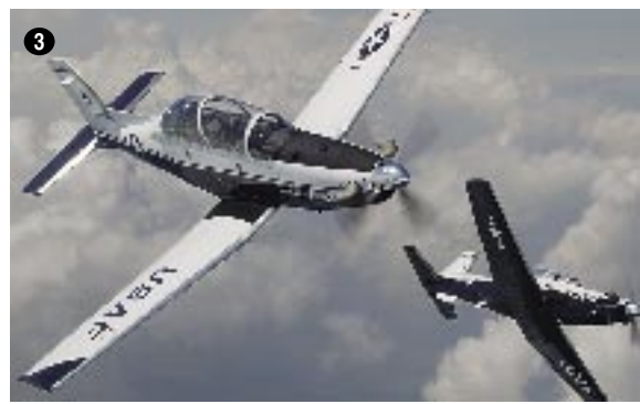
[3] Two Texans reveal the white-on-blue paint scheme, meant to enhance visibility while reducing maintenance.
