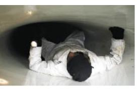
The white-clad airman above is entering the air intake of an F-16 to check for engine blade damage.
