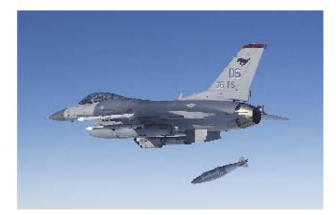
The F-16 at right has just released a 2,000-pound satellite guided GBU-31 Joint Direct Attack Munition. The Air Force is counting on such precision guided weapons to counter the vast North Korean military. Global Positioning System accuracy means that JDAMs are unaffected by the frequent clouds and rain on the Korean Peninsula.
