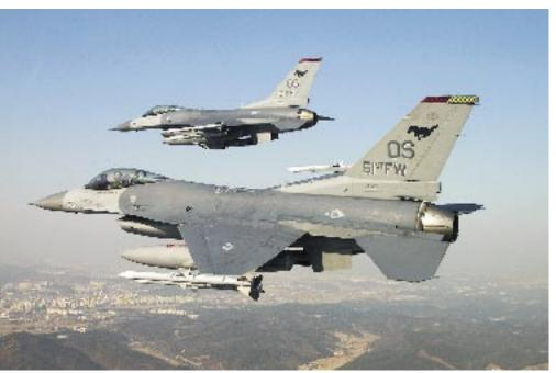
A pair of F-16s patrol South Korean skies near Seoul. In the foreground is the 51st FW's flag aircraft. The F-16's versatility is illustrated by the AIM-120 AMRAAM missiles that offer beyond-visual-range air-to-air capability and the large, external fuel tanks that extend the aircraft's range and endurance.
