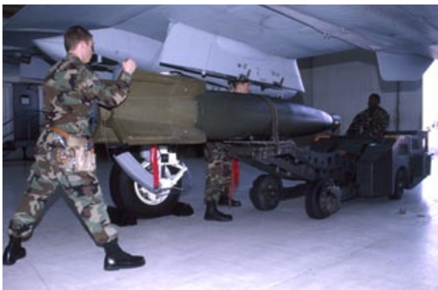
In the top photo, SrA. Rodney Groom of the 357th Fighter Squadron at Davis-Monthan brings an AGM-65 Maverick missile out of its container for a weapons-load demonstration. Photo above shows a TV-guided Maverick installed on a wing pylon.
