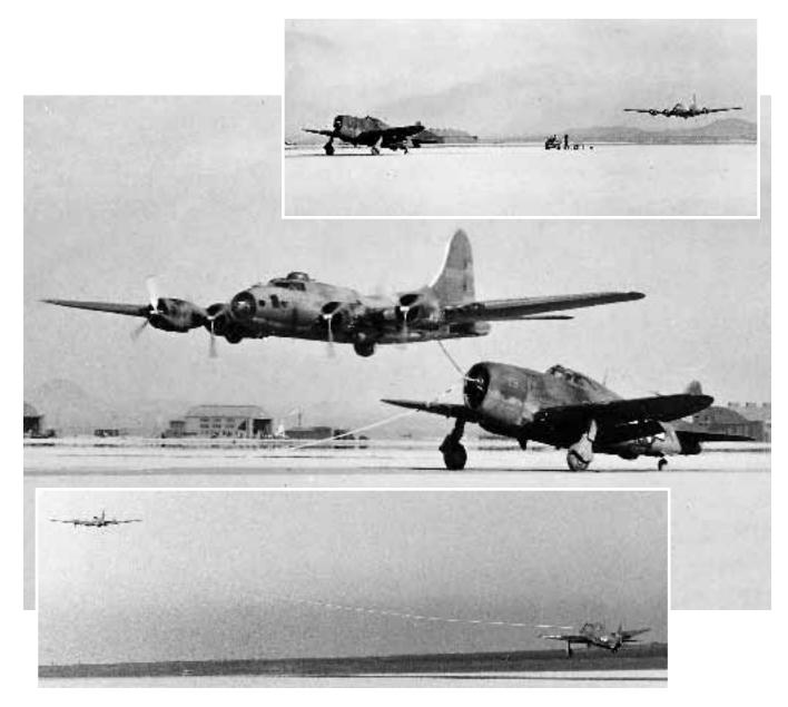
US Army Air Forces of World War II hated to lose a serviceable fighter aircraft just because mechanical problems might force it to land in an inaccessible spot. To solve the problem, USAAF's Equipment Laboratory at Wright Field, Ohio, experimented with airplane snatching, seen in this photo sequence in which (top to bottom) a B-17 bomber scoops up a P-47 fighter. First, a tow bridle was attached to the fighter. Then, two upright poles were planted, with the bridle's pick-up loop strung across
