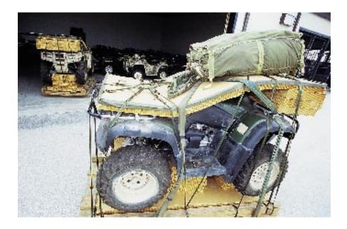
Everything needed for rescue must be ready to go at a moment's notice. At left, all-terrain vehicles are packaged with parachutes, prepared for a combat drop, mounted on shock-absorbing material that will cushion the jolt of a landing on hard ground. The PJs themselves are responsible for keeping their Zodiac boats, medical gear, and weapons in top condition and primed for action, but support personnel have recently been made available to tend to the equipment while the PJs are "on assignment."
