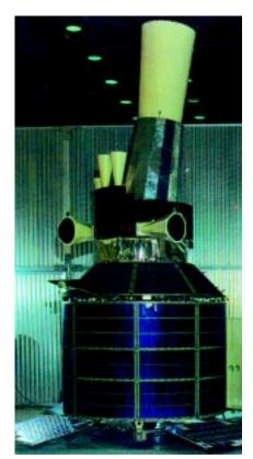
A DSP satellite, with infrared sensors that provided space-based early warning of missile launches.
