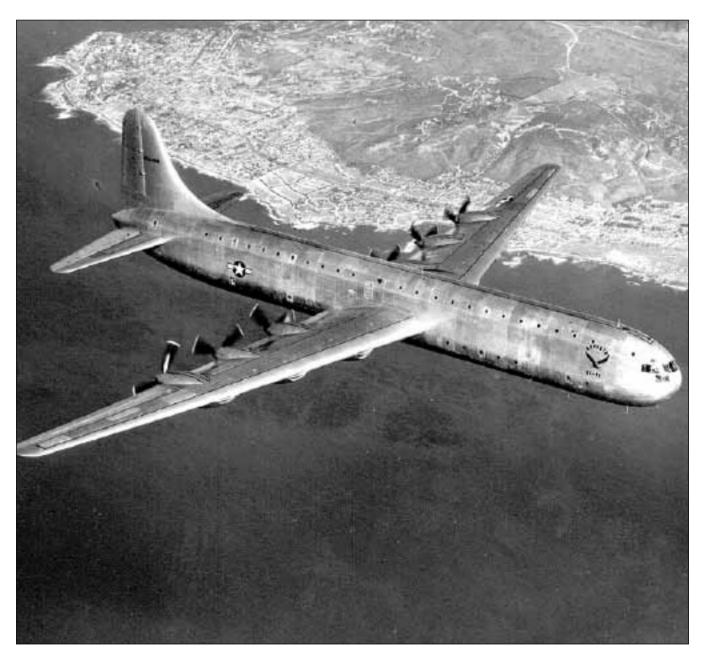
The 1947 press release from Consolidated Vultee Aircraft Corp. proclaimed this XC-99 transport—shown in flight off southern California—as "the world's largest land plane." It was 182.5 feet long and 57.5 feet tall—longer and taller than its sister aircraft, the B-36, though they both had a 230-foot wingspan. The XC-99 had two levels of cargo decks. Its interior volume equaled that of 10 railroad freight cars, and it could
