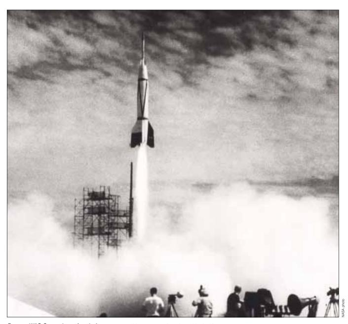
Bumper–WAC Corporal was America's first large two-stage rocket. It was a German V-2 topped with a US Army Corporal missile. Eight such Bumper–WACs were assembled. The first launch took place on May 13, 1948, at White Sands Proving Ground, N.M. The hybrid system attained only slightly more speed and altitude than a V-2, but on Feb. 24, 1949, a Bumper–WAC set records for a man-made object,
