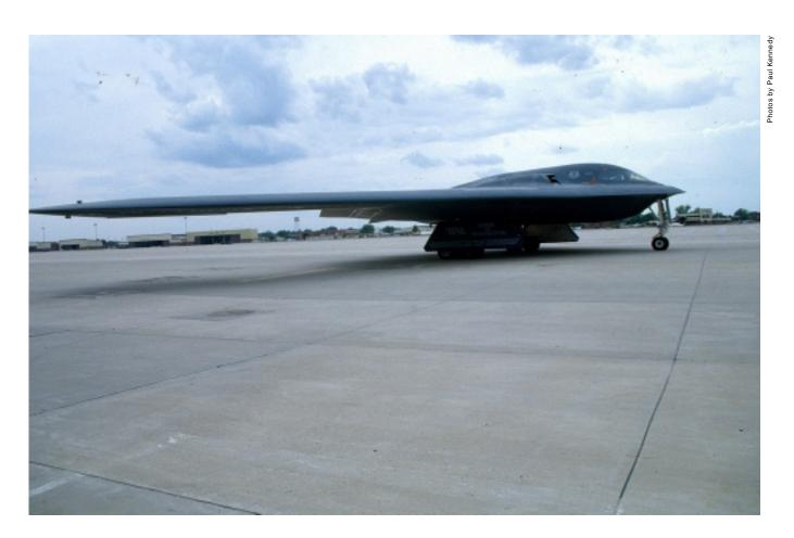
The B-2 Spirit is 17 feet high and 69 feet long, with a wingspan of 172 feet. Above, one of the huge landing gear doors bears the tail code for this tailless aircraft. Intakes show where air enters for the four engines buried deep inside the wing. At right, a back view shows where and how the exhaust is ducted to help reduce the B-2's signature.
