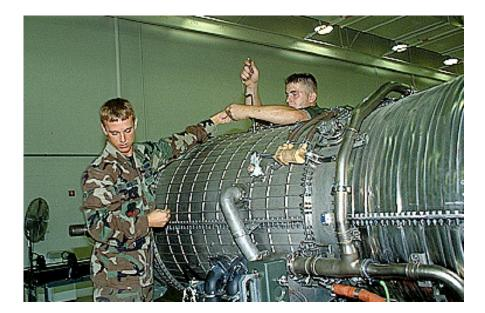
The B-2 is powered by four GE F118-GE-100 turbofans, each with more than 17,000 pounds thrust. It can carry a payload of more than 40,000 pounds and has an unrefueled range of more than 6,000 miles.
