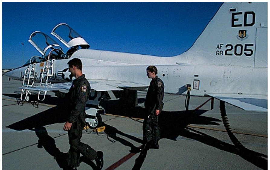
At right, Dutton and Dale go over details with the ground crew and perform their walk around check. They are going to fly a Data Acquisition System T-38. It's been modified with data collection equipment, including the test pitot tube mounted on the nose (top right). The idea is for the students to fly the jet and collect data, as if they were testing a new aircraft.
