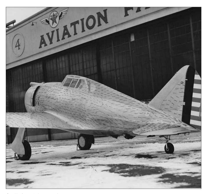
Searching for ways to improve aerodynamic design, engineers had one side of this new Republic P-43 Lancer covered with pieces of string. The engineers then used movie cameras to record movements of the strings during wind tunnel and other tests. In this way, they determined the patterns of airflow over different parts of the aircraft.
